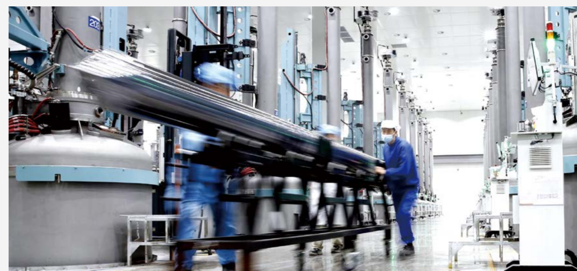
Xuzhou Photo voltaic Granular Silicon Technology Application Demonstration Project. Employees are transporting a 6-meter-long monocrystalline silicon rod.
